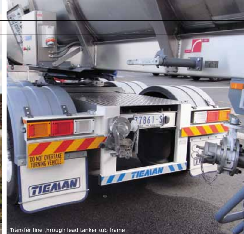
Transfer line through lead tanker sub frame
