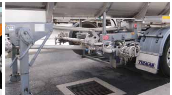
Transfer line through lead tanker sub frame
