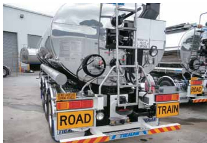
Hinged rear ladder allowing Ringfeder connection to dolly and safe entry to top walkway
