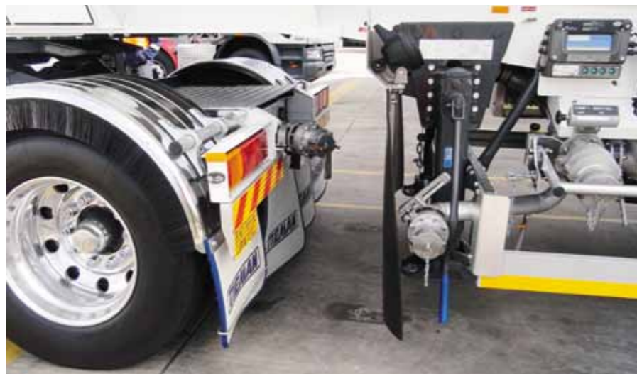
A short transfer hose is used to suck fuel from the dog trailer.
