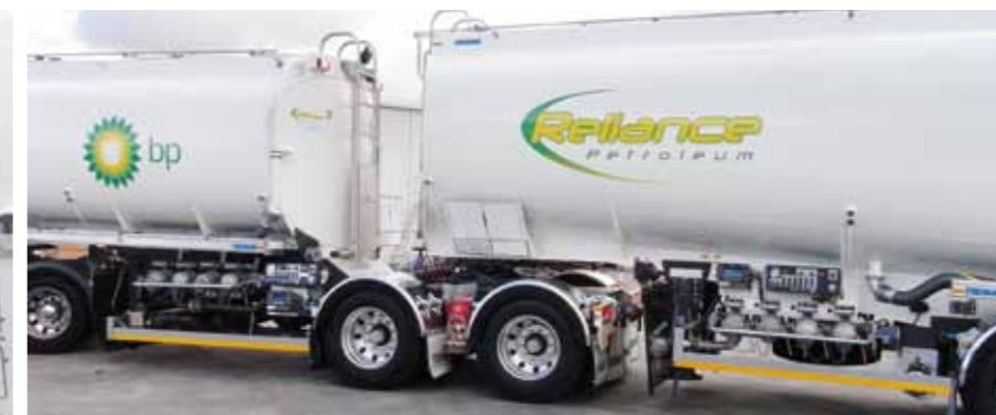
Side under run protection with transfer line from lead tanker outlet area running through the suspension sub frame terminating at rear of sub frame.
