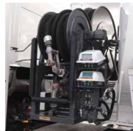
Front of tanker mounted hose reels are protected from road grime and operated from shoulder height with no back bending required.
