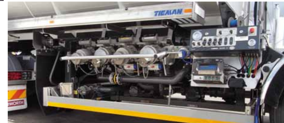
Pipe work on the four compartment lead tanker exits through the sub frame to optimise API valve heights for easy gantry loading.
