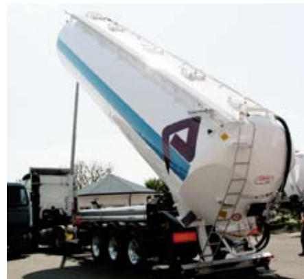
Lightweight full aluminium subframe.
