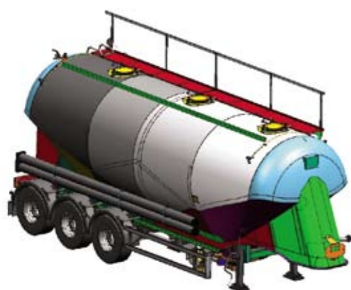
A dry bulk tanker in Solid Works 3D, the software both O.ME.PS and Tieman use to design tankers. Clients can view the design prior to the start of the building process.
