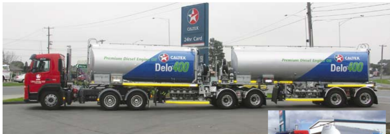
The Tieman 'Split Shifter' carries several thousand litres more diesel than a rigid and dog trailer
