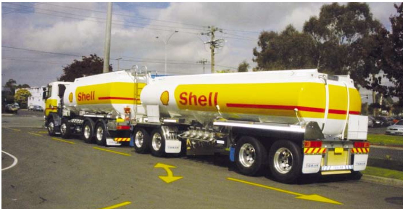
Tieman's 20,000-litre, 8x4 rigid 'DirtEdog' tanker for Shell.
