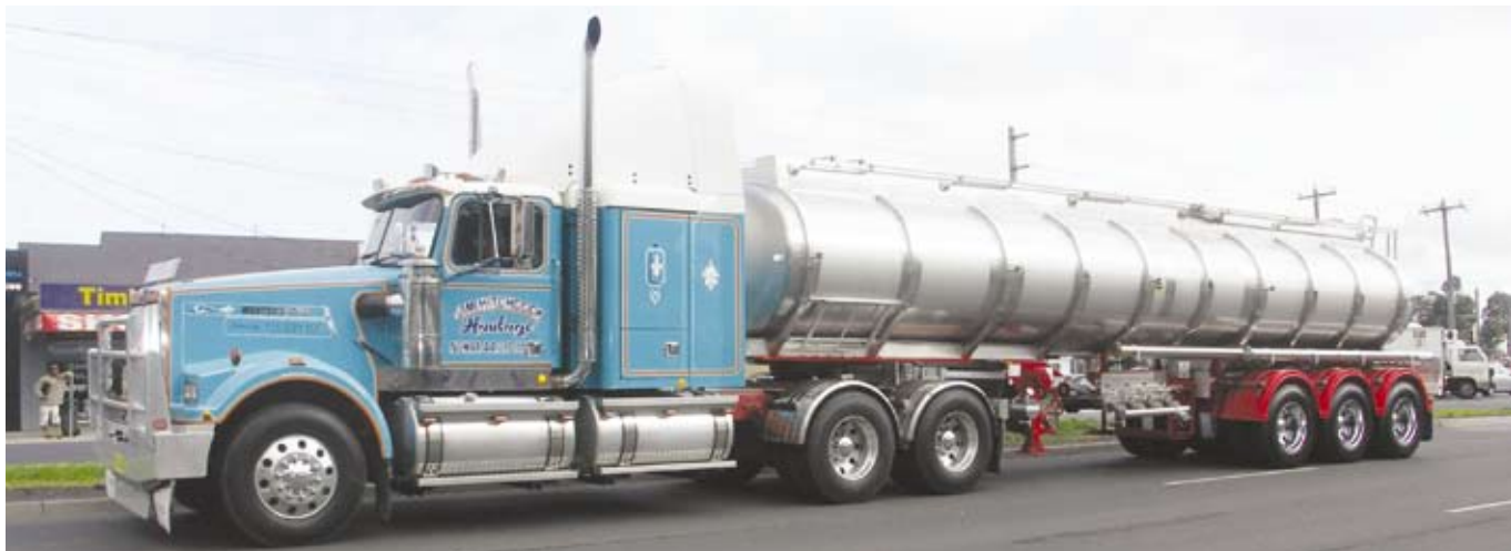
A Hitchcock Haulage 28,000-litre, four-compartment Class 8 stainless steel chemical tanker.
