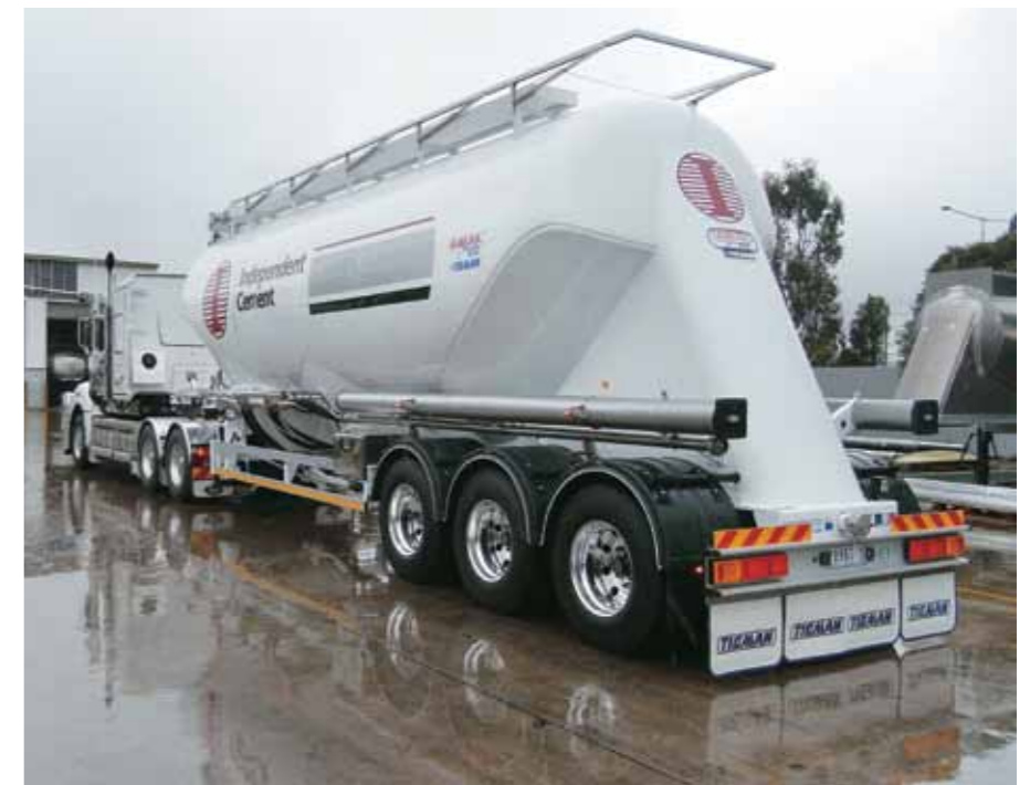
Polished stainless steel airlines & side under run protection
