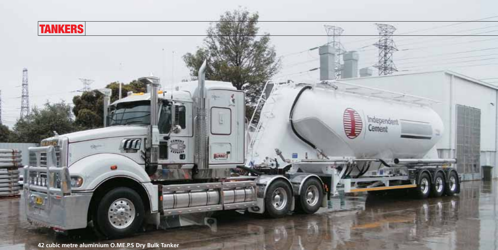
42 cubic metre aluminium O.M.E.P.S Dry Bulk Tanker
