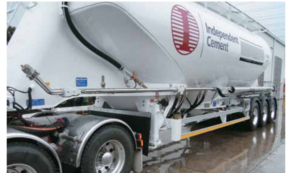
Polished stainless steel airlines & side under run protection
