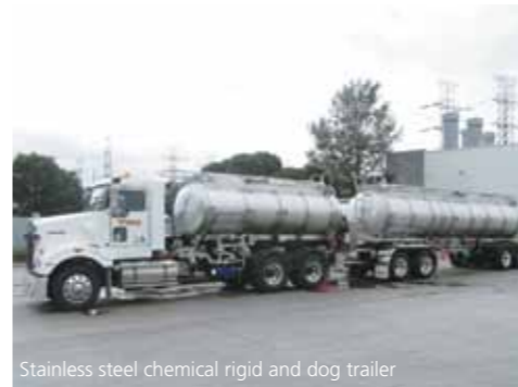
Stainless steel chemical rigid and dog trailer
