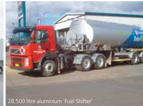
28,500 litre aluminium 'Fuel Shifter'
