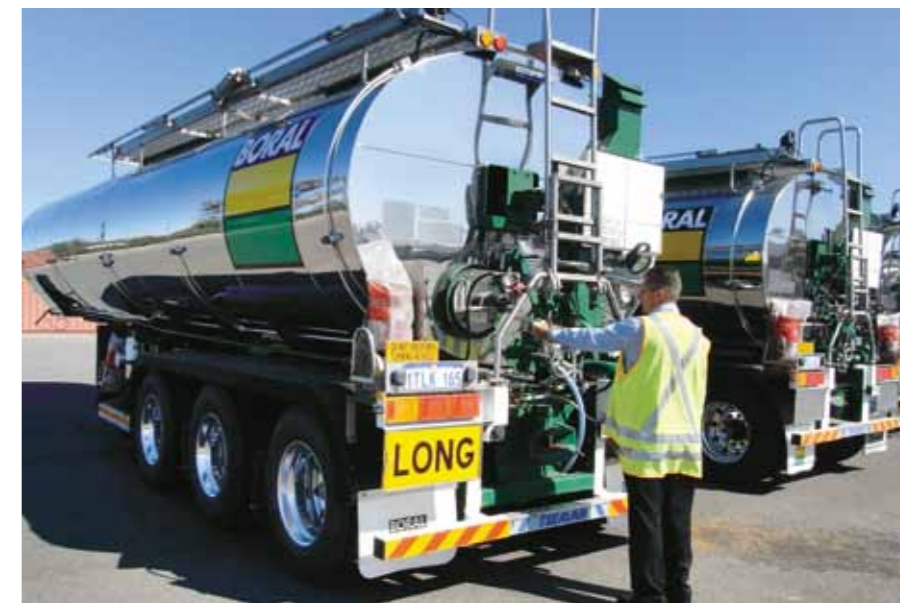
New Tieman Safety Feature – rear pump control handle operated from ground level
