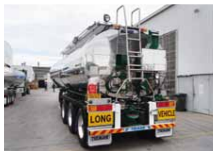
Hinged rear ladder interlocked with the top handrails.
