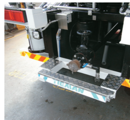
Hinged rear bumper for easy spill bucket positioning.
