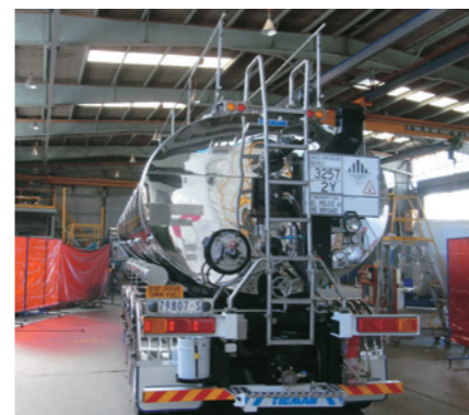
Lowering ladder automatically raises handrails and applies brakes.
