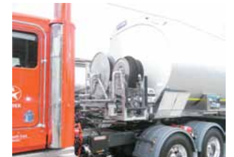
Hose reels mounted off front of tanker, operated from shoulder height.
