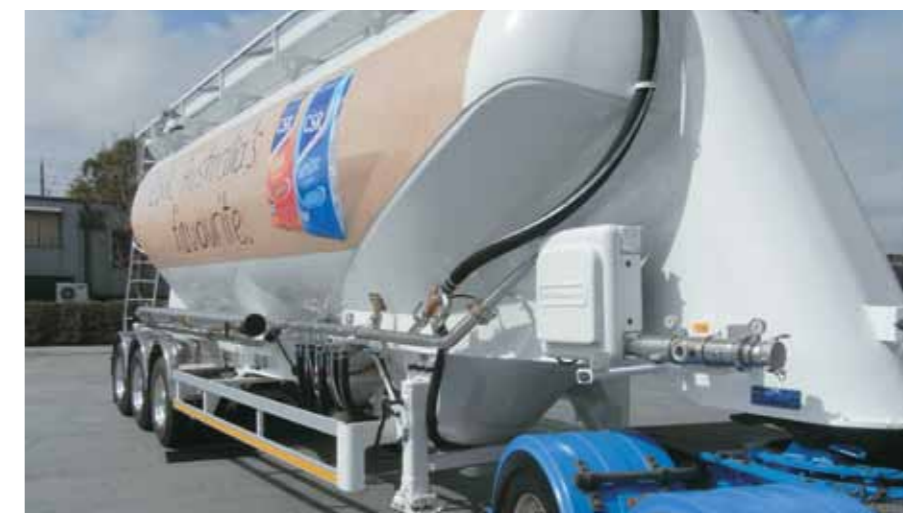
Polished stainless steel airlines, in line filter, drum air cooler and side under run protection.
