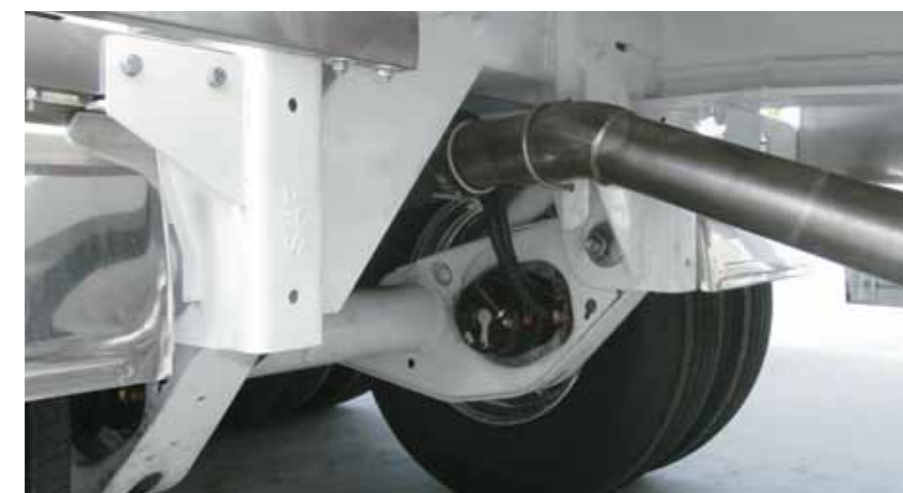
Bolted steel hangers & stainless steel discharge pipes.
