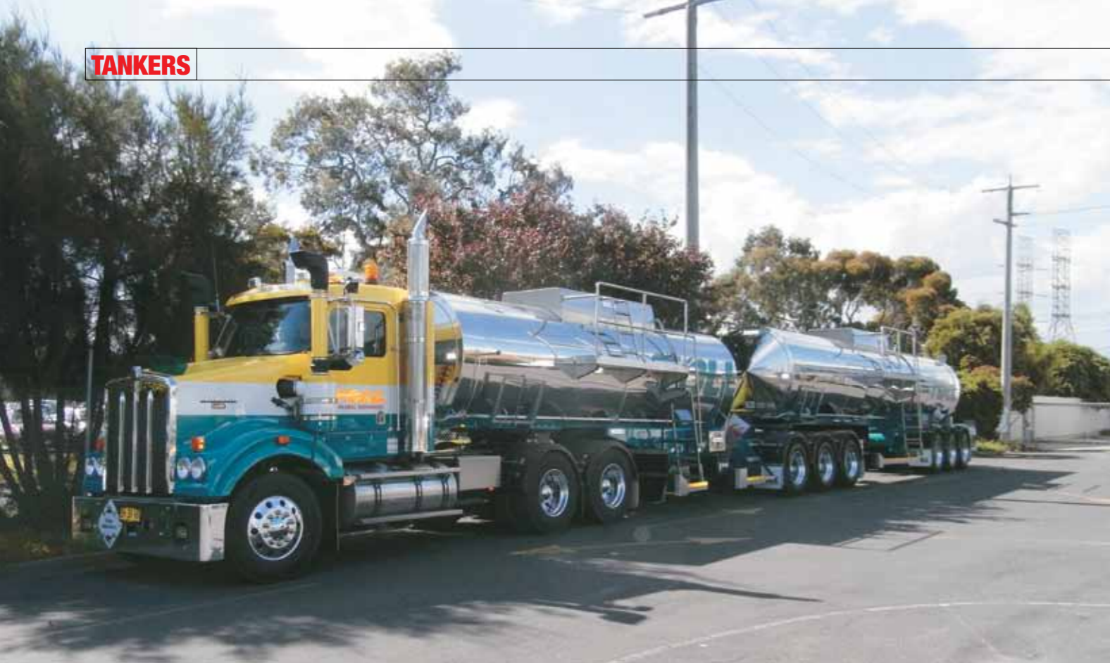
Tieman 25m B-double ammonium nitrate solution combination.
