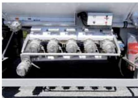
Tieman manifold allowing quick discharge at mine sites.
