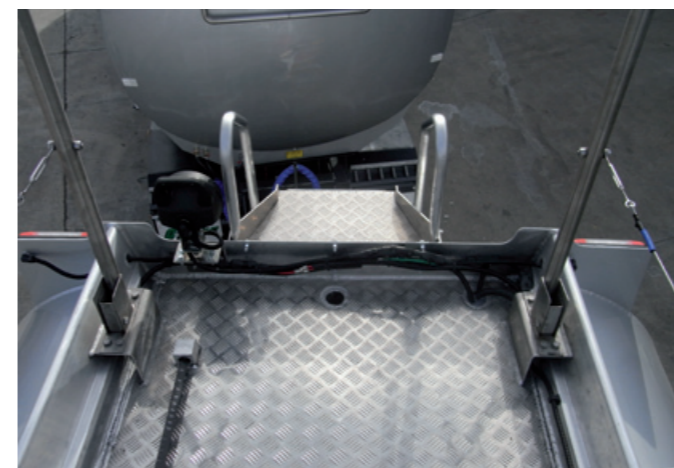
Another safety feature: Tieman's safe exit platform to the top of the ladder.
