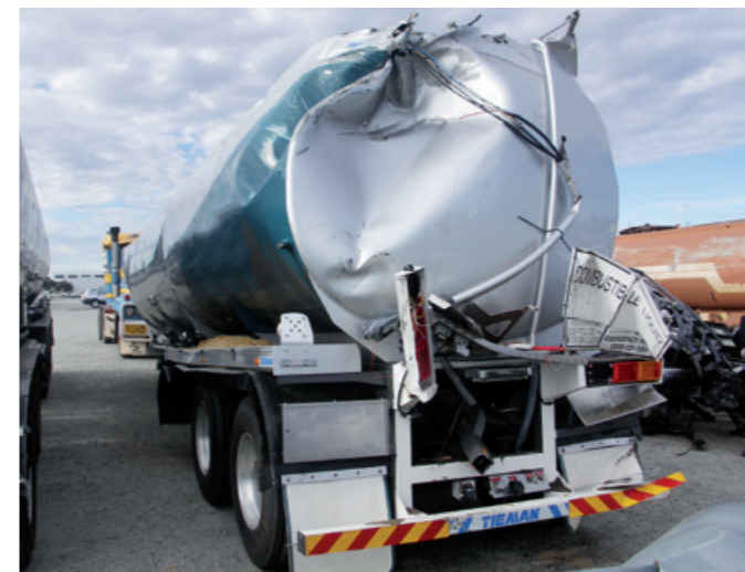
Major rollover - Only one compartment of fuel lost due to compartment rupture.
