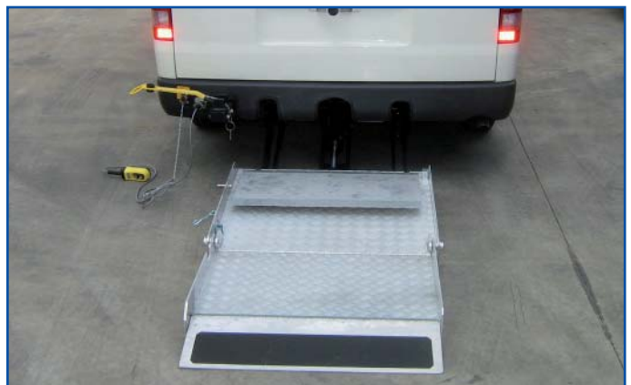
TD350A fitted to van in fully lowered position.
