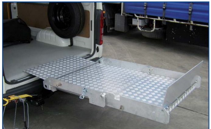
TD350A fitted to van at vehicle floor position.
