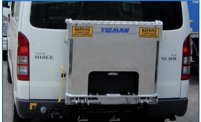
TD350A fitted to van in stowed position.
