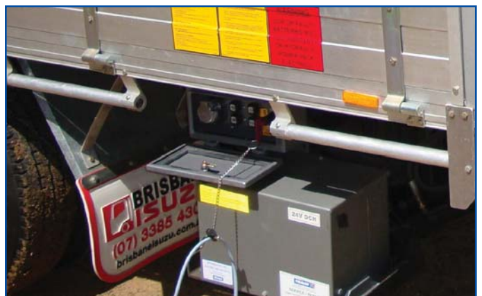
Safe operating instructions, enclosed power pack, lockable control box.
