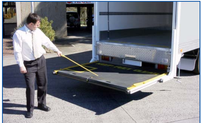
TR1000S platform manually deployed from stowed position ready for use.
