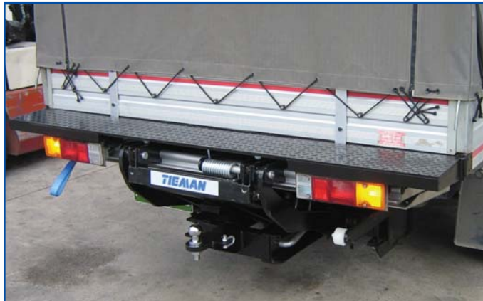
TK505 AL shown in stowed position with optional extra tow bar attachment fitted.
