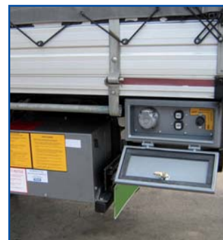
Safety & operating instructions, enclosed power pack and lockable side control box.
