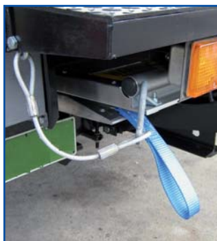
Platform stowing cable & hasp and heavy duty blue hand straps for assisting platform opening/closing function.
