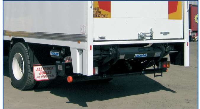
Platform stowed away.
